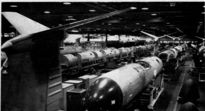
A steady stream of TM-76 Mace missiles rolls off the production line at the Baltimore plant of the Martin Co. The all-weather cruise-type birds are being assembled at Sembach to replace the Matador in Wing units.
